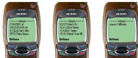
Figure 3: Example of an SMS message automatically sent for the system check status.
