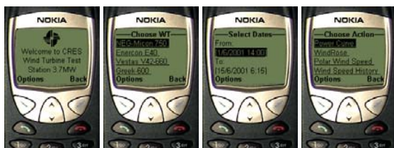
Figure 5: Example of a navigate through the menu of the CRES Wind Farm, WAP communication system.
