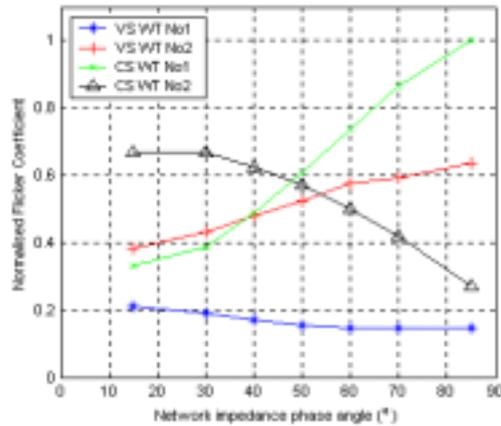
**Figure 2:** Flicker coefficients as a function of network impedance phase angles for the all the WTs.
