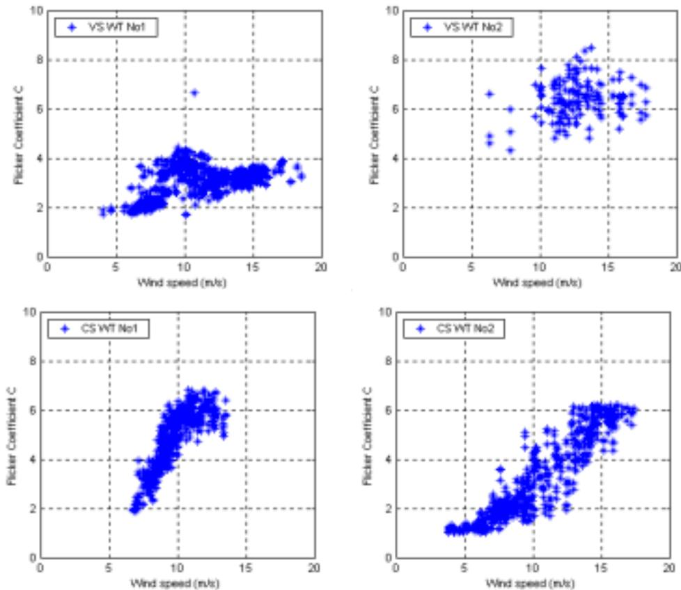
**Figure 3:** Flicker coefficients as a function of wind speed for all the WTs
