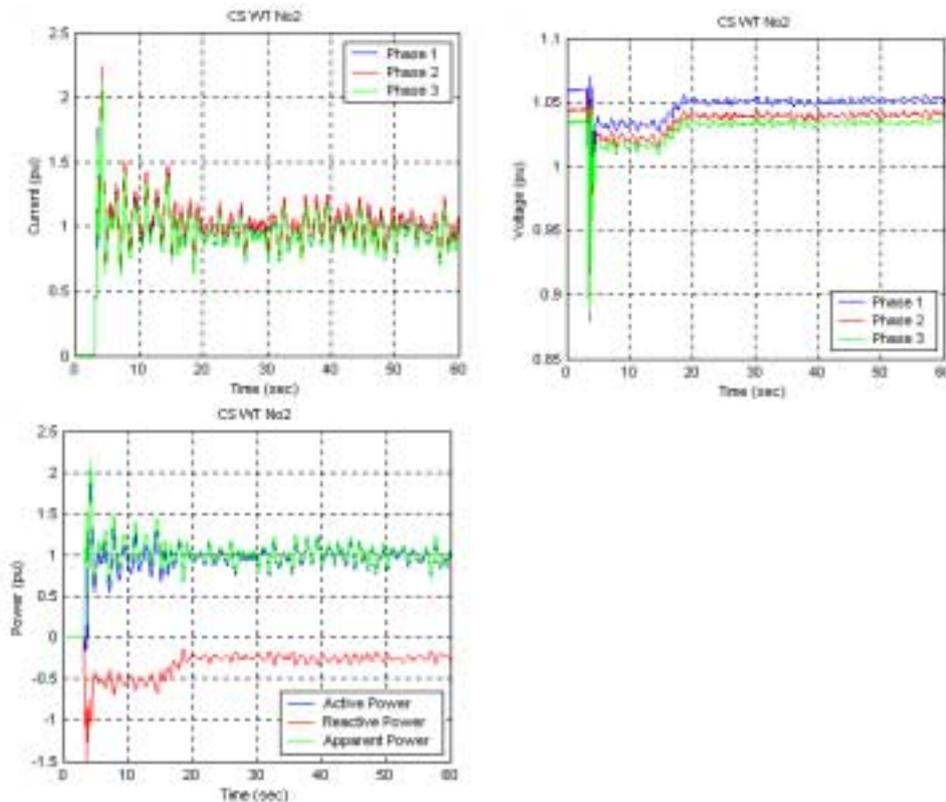
Figure 5: Constant speed wind turbine start-up at rated wind speed
