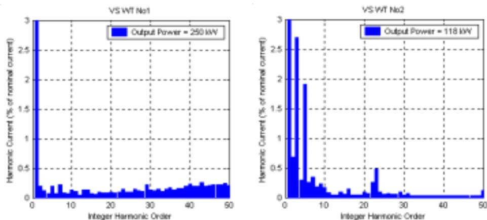
**Figure 7:** Phase-1 integer harmonic amplitude of the variable speed wind turbines
