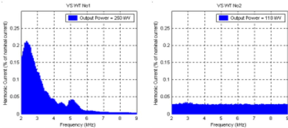
Figure 9: Phase-1 integer and inter-harmonic currents from 2 to 9 kHz for the variable speed WTs
