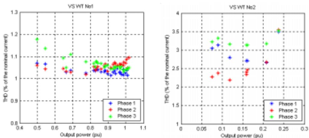
Figure 10: Total harmonic distortion as a percentage of nominal machine current vs active power for the variable speed WTs
