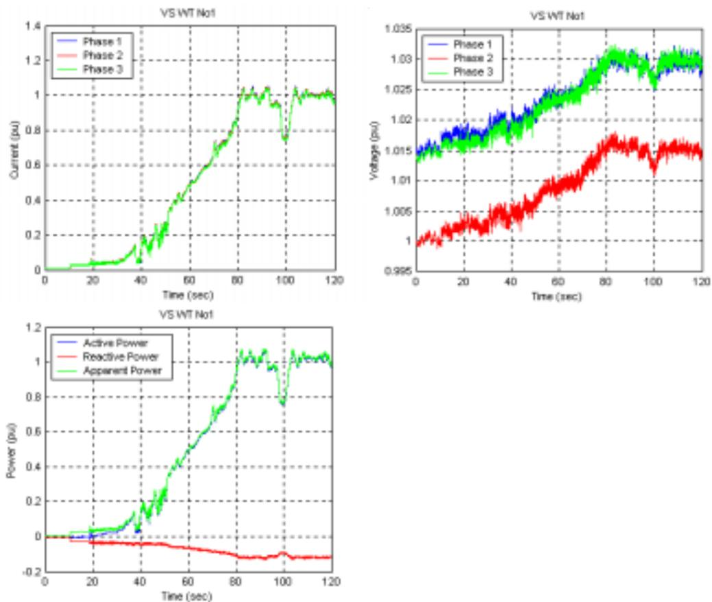
**Figure 6:** Variable speed wind turbine start-up at rated wind speed
