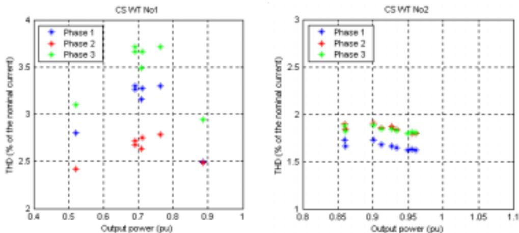
**Figure 11:** Total harmonic distortion as a percentage of nominal machine current vs active power for the constant speed WTs
