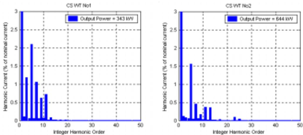
Figure 8: Phase-1 integer harmonic amplitude for the constant speed WTs
