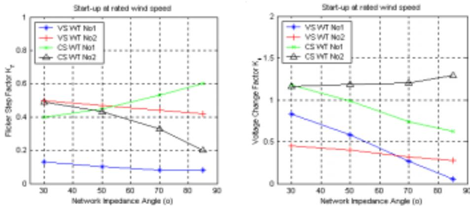
Figure 4: Flicker Step Factor and Voltage Change Factor for each WT, as a function of network impedance phase angles
